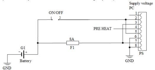
GND is connected to the vehicle's ground.
