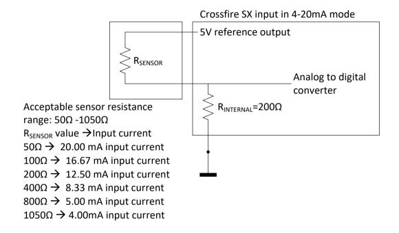
As shown in the figure there is an internal 200 resistor connected to ground in Crossfire SX when the input is configured for 4-20mA current input. The sensor resistance can be calculated from the current reading according to:
