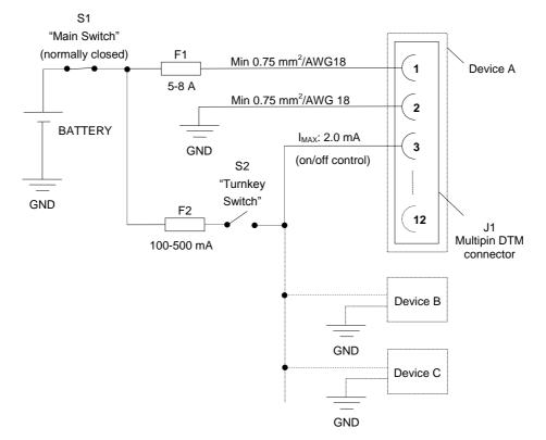
Schematic example for power supply installation of one or more *CCpilot* VA devices in vehicles or other machines. The on/off control switch (S2) is shared by several devices (Device A, B, C...).
