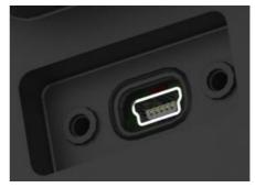
Note: The ID-pin is used for selecting USB host-mode (pin low) or USB device-mode (pin high/floating). By default, the ID-pin is held low internally from CPU I/O-pin to force USB host-mode operation.
