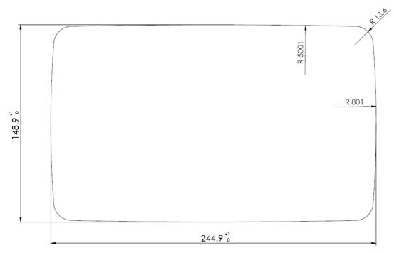
The device has a built-in gasket to provide some amount of sealing towards the panel. Ensure that the device is mounted to a smooth, flat surface. Fastening the device to an uneven surface will affect the sealing property and may stress the enclosure or damage the outer flange, leading to premature failure. Additional gasket or other means for sealing may be required to reach higher IP levels.
