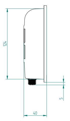
Mount using a RAM mount (i.e RAM-202U) or panel mounting bracket C000152-48).
