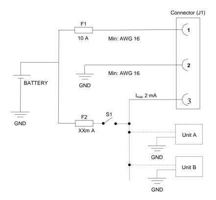
By connecting the power supply according to the illustration above, the device will automatically start when the main switch or turnkey is turned on, and shut down when the switch or turnkey is turned off.
