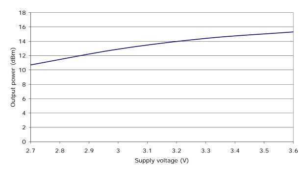
Figure 4: WT11 output power vs supply voltage
