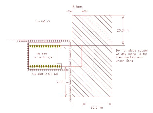
Figure 30: Suggested PCB design around ACX antenna with the module et the edge of PCB
