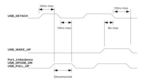
Figure 13: USB\_DETACH and USB\_WAKE\_UP Signal
