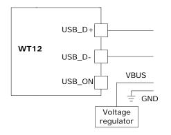
Figure 12: USB in bus powered mode
