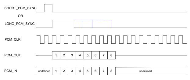
Figure 18: Multi Slot Operation with Two Slots and 8-bit Companded Samples
