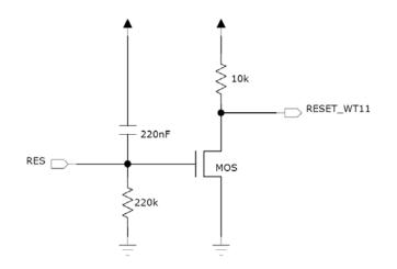
Figure 6: WT11 internal reset circuitry
