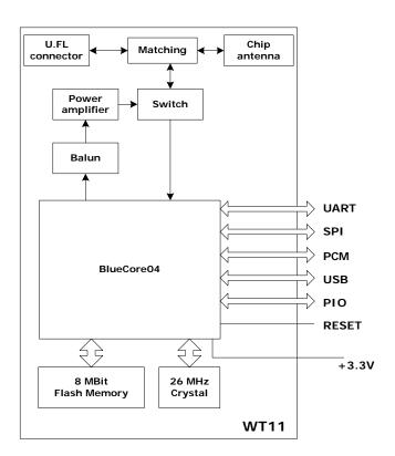
Figure 3: Block Diagram of WT11
