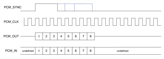
Figure 16: Long frame sync (shown with 8-bit Companded Sample)
