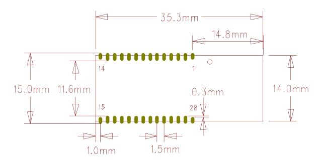
Figure 33: WT11 foot print and dimension (top view)
