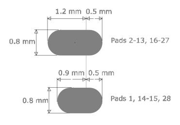
Figure 34: WT11 pad dimensions
