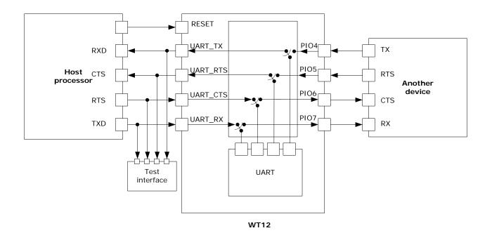
Figure 10: UART bypass mode
