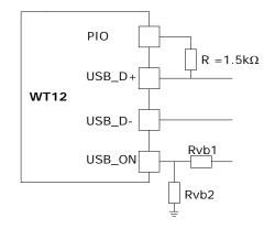
Figure 11: USB in self powered mode
