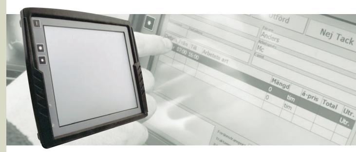
The **CC Pilot XS All-Integrated** is a powerful, versatile and robust on-board computer for use in control systems and Fleet Management applications. With its rich set of features it functions as the central component in a totally integrated mobile system. The CC Pilot XS All-Integrated is an industrial product, intended for heavy duty professional use.
