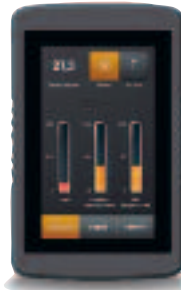
The new concept for maximatecc operator panels uses a 4.3" PCAP touch screen, enabling a Smartphone-like user experience
