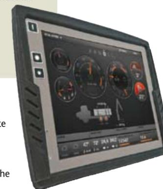
XLS, thereby ensuring the integrity of all parts of the display computer. The power supply within the unit is managed by this CPU. In a safety-critical system it is essential that power is managed in a way that ensures safe states at all times. Monitoring of internal temperatures, supervision of internal oscillators and control of the display backlight is also carried out in this CPU. In addition, the system supervisor performs sequence checking – a very important aspect in safety systems.
