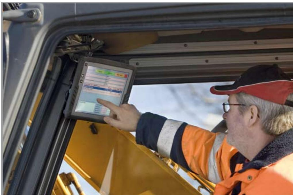
FIGURE 1: Safe display computers are needed in industrial vehicles
