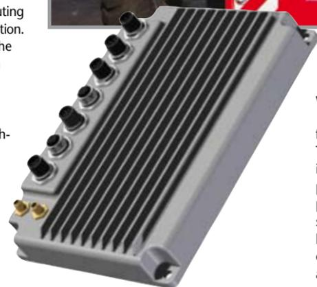
gateway between the different networks. To facilitate the integration of non-CAN subsystems, the platform has Ethernet as well as host and device USB interfaces.
