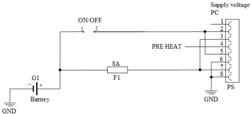
GND is connected to the vehicle's ground.
