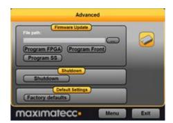
Each of these firmware components can be updated, either individually or batched. The preferred method to perform the update is by using the *CCSettings* program, as briefly mention in section **Error! Reference source not found.** It is also possible to use the command line based application *ccsettingsconsole*, or from your own program using the CC AUX API functions.
