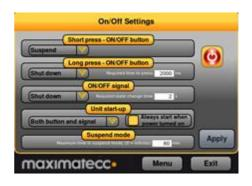
*ON/OFF signal* - adjust the behavior of the On/off signal through the power connector. The time settings adjust how long the signal must stay low before XM2 device reacts to the signal.
