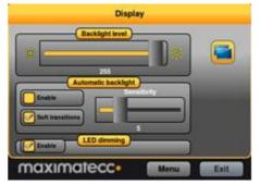
The *Sensitivity* slider adjusts the level and phase of backlight adjustment depending on the surrounding light.
