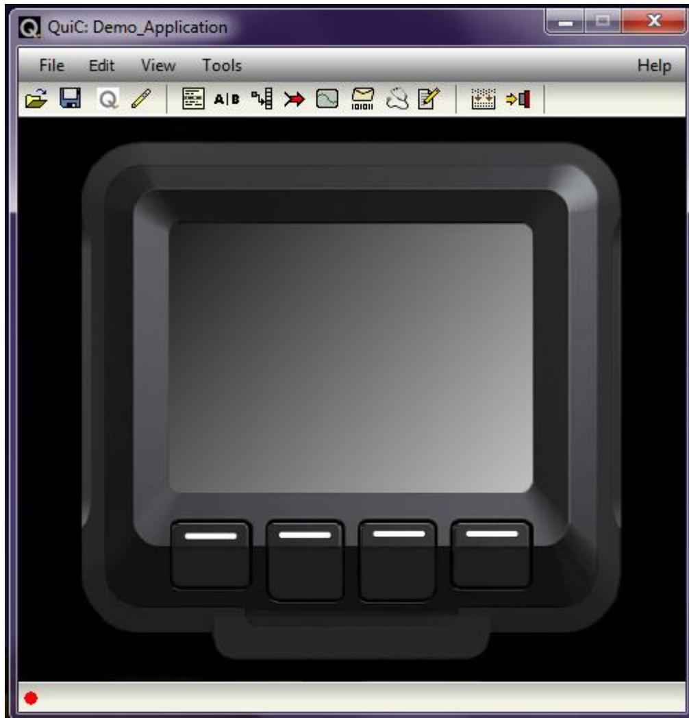
For navigation to the ['Screen Designer'](#) and ['Layout Designer'](#), move your mouse onto the screen of the digital CCPilot VI display pictured in the tool until there is a yellow dotted line around the screen. Now click the mouse.
