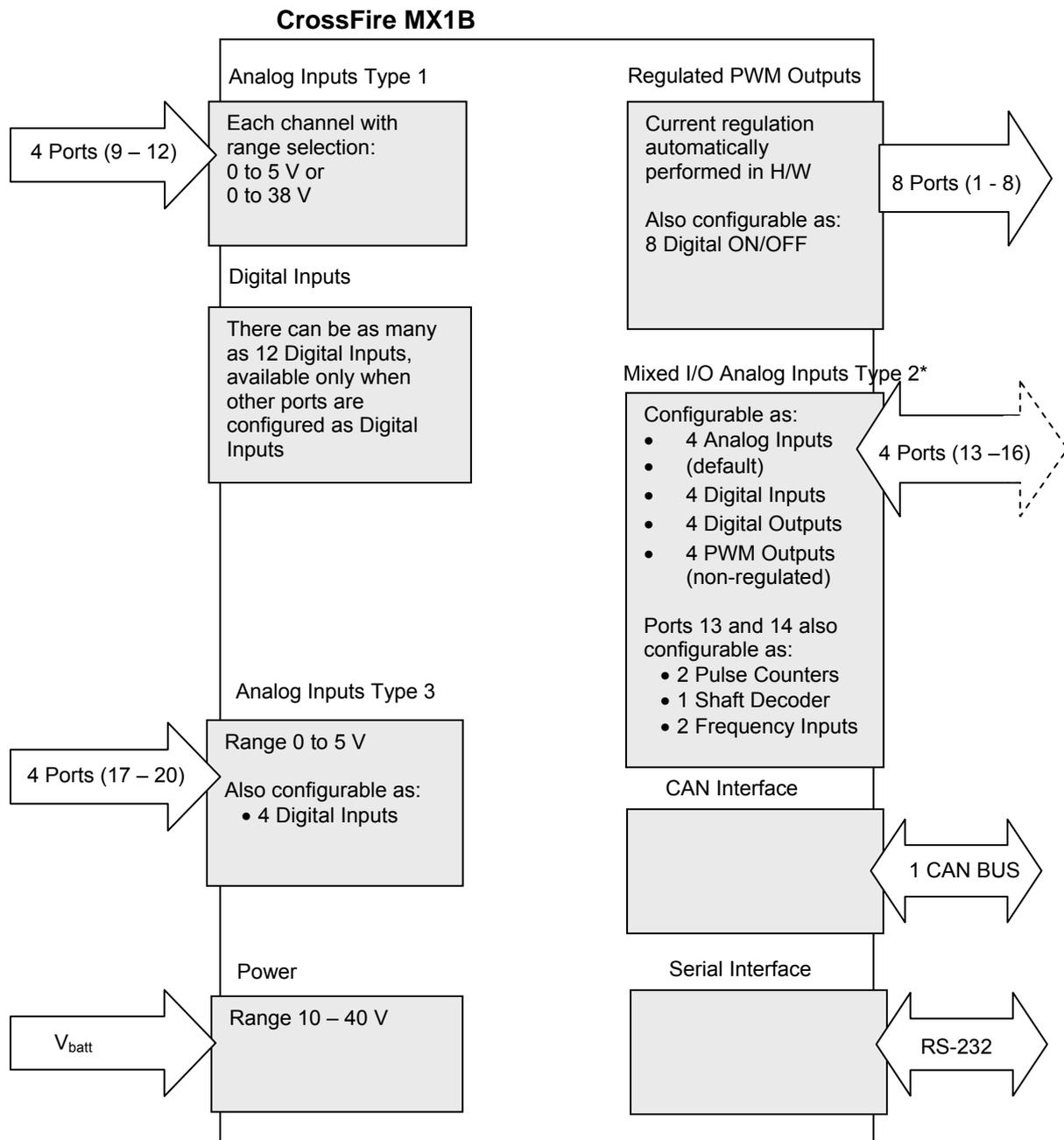
\* The analog inputs that are combined with on/off outputs shall only be used as feedback for the outputs. Because of the open-load detection feature there will be a low current flowing to these outputs. This makes the inputs not useful as ordinary analog inputs.
