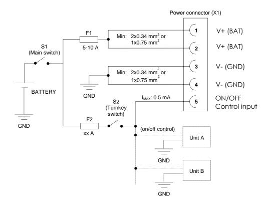
Schematic example for power supply installation of *CCpilot XA/XS* and *CrossCore XS* devices in vehicles or other machines. The on/off control switch (S2) is shared by several devices (Unit A, Unit B etc.).
