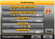
*ON/OFF signal* - adjust the behavior of the On/Off signal through the power connector. The time setting adjust how long the signal must stay low before the device reacts to the signal.
