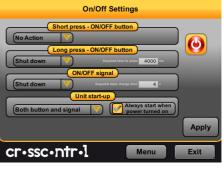
*Long press - ON/OFF button -* adjust the unit behavior when pressing and holding the On/Off button.
