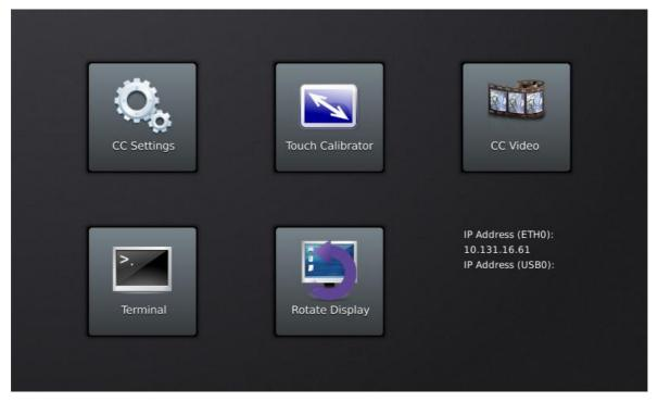
A user can and should replace or simply edit the default startup application script, i.e. the init script found at /opt/etc/init.d/StartupGui. This init script is automatically run when entering run level 3 (during boot) or run level 6 (during shutdown/reboot).
