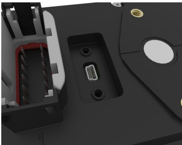
Note, the sealing property of the unit is affected when accessing the second USB port located under the hatch.
