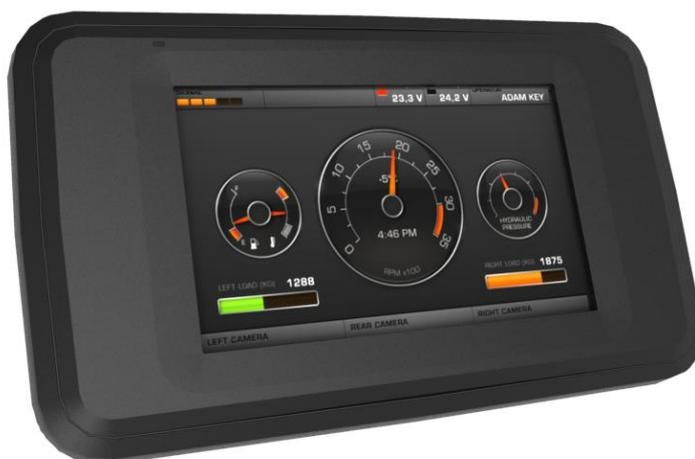
On the rear side of the device are the interface connectors (Deutsch DTM-12) and a USB connector located under a cover. There are also mounting holes for fasteners in accordance with AMPS hole pattern (RAM 2.43" x 1.31" Diamond Base) or bracket for panel mounting.
