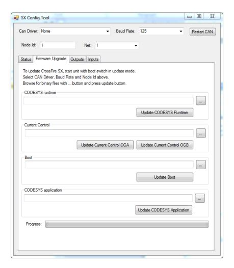
Click on the "…" button in the CODESYS runtime area of the window. Browse to the location of the SX\_CODESYS\_x\_x\_x\_x.bin file, select it, and click Open. The file path should be shown in the CODESYS runtime area of the window.
