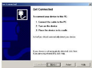
When the dialogue *Get Connected* is shown, the following steps must be carried out so that a connection can be established with the CC Pilot<sup>™</sup> XS:
