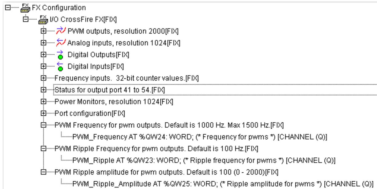
Under the I/O tree structure it is possible to access all I/O through variables. The variables are global and can thereby be accessed in all your code modules. It is also possible to change the names of the variables by clicking on them and writing a new name. For example, below, Port 61 which is a PWM output has been given the name MotorSpeed:
