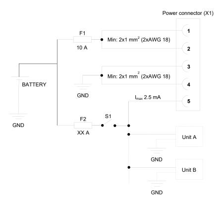
By connecting the power supply according to the illustration above, the device will automatically start when the main switch or turnkey is turned on, and shut down when the switch or turnkey is turned off. While the main switch is in the ON position, the computer can also be turned off and on with the On/Off-button.
