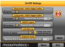
*ON/OFF signal* - adjust the behavior of the On/Off signal through the power connector. The time setting adjust how long the signal must stay low before the device reacts to the signal.
