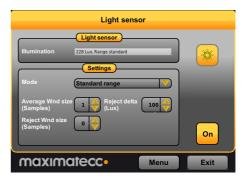
If the difference of the maximum value and the minimum value in the number of samples in the reject delta window is larger than the reject delta, those samples are discarded.
