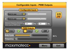
choose PWM1 or PWM2 in the radio button and adjust its parameters from the sliders below.
