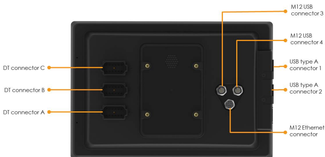
Figure 7: CCpilot VS 12" connectors
